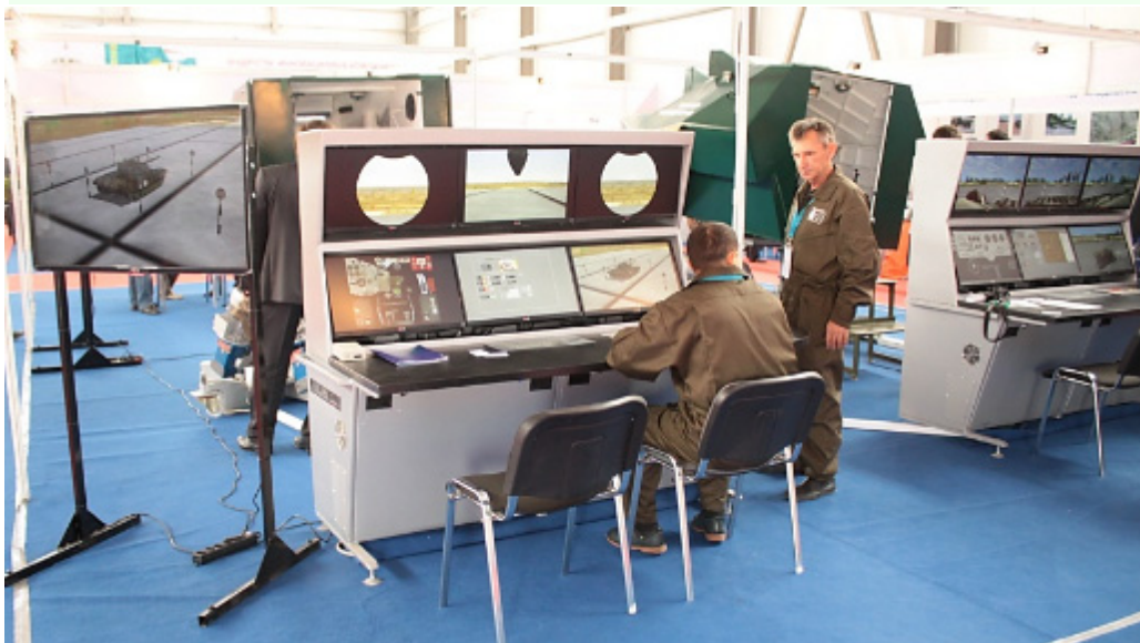
External controllable camera view display at the Instructor's work station
