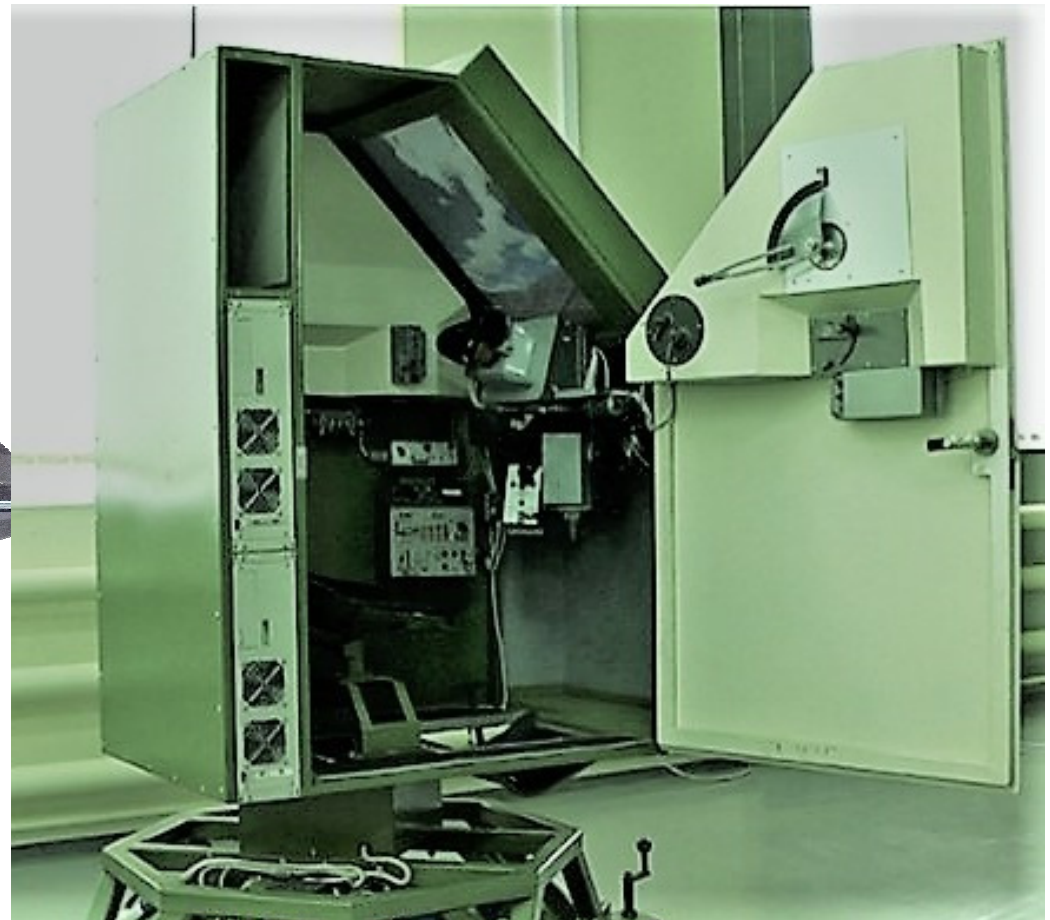
The general view the functional turret mock-up mounted on a circular rotation platform
