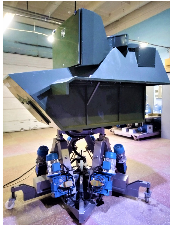
General view of driver's cabin mock-up mounted on 6DOF motion platform
