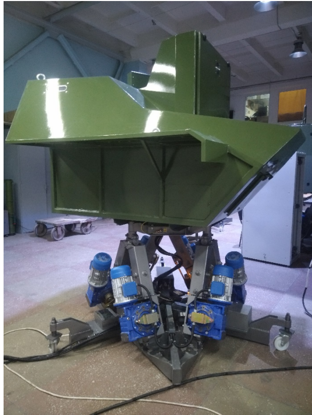
General view of driver's cabin mock-up mounted on 6DOF motion platform
