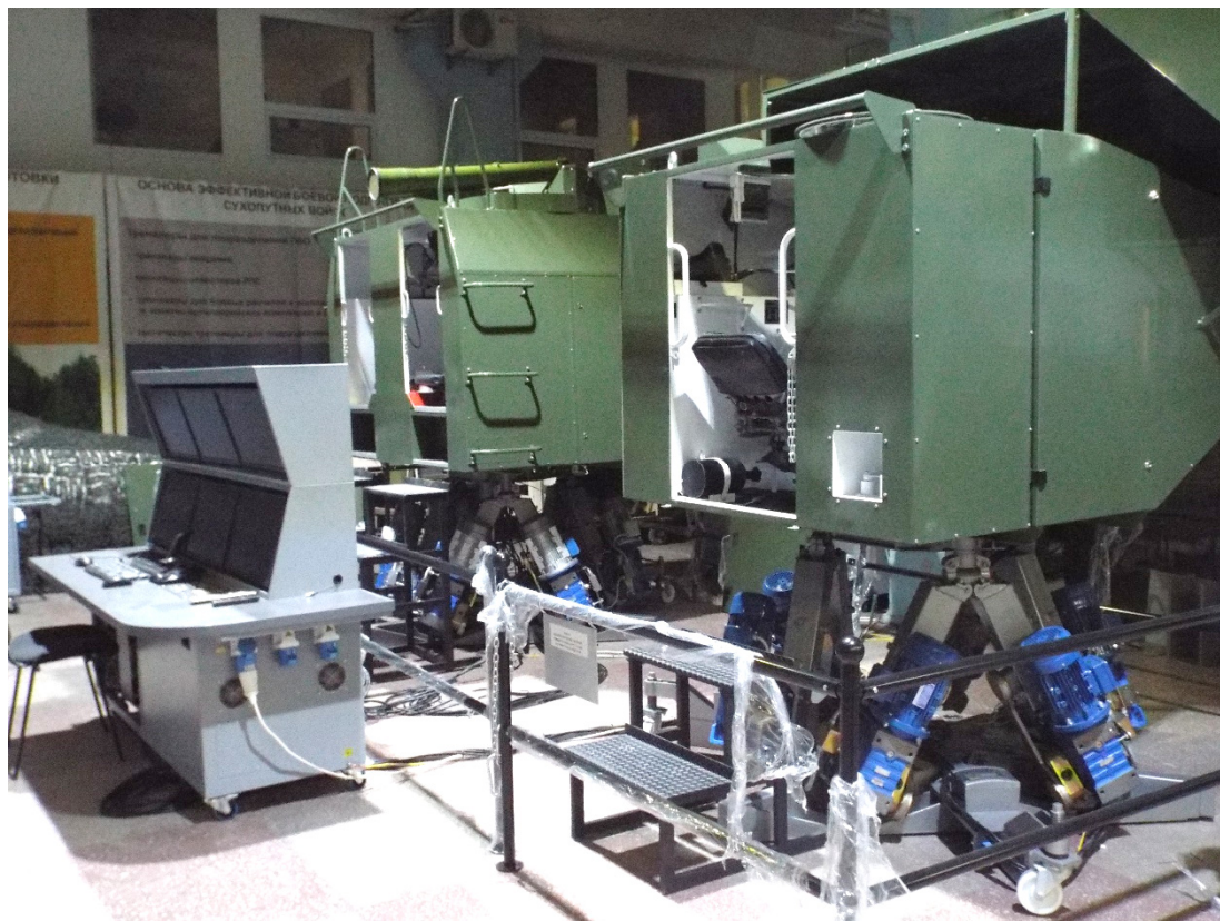
View of BMP-2 driving cabin mounted on 6-DOF dynamic platform
