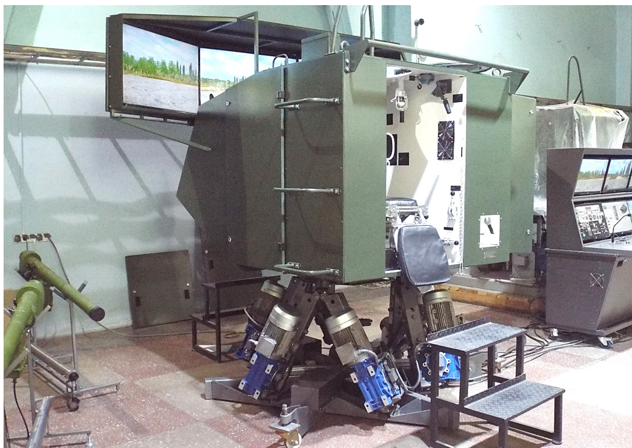
View of BMP-2 driving cabin mounted on 6-DOF dynamic platform
