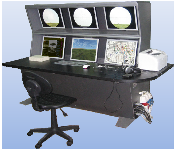
Instructor's workstation with software and hardware suite and operator's workplace
