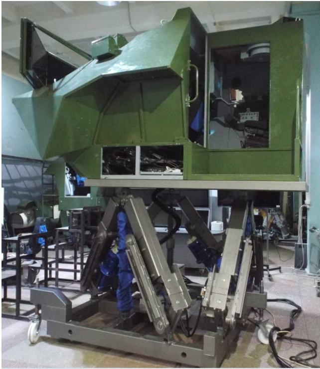
General view of integrated BTR-3E1 crew simulator
